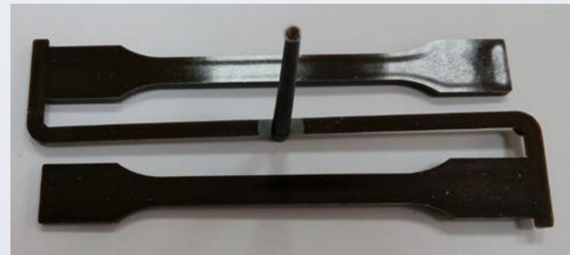
Biocomposite compact (used coffee grounds 45% by weight)
