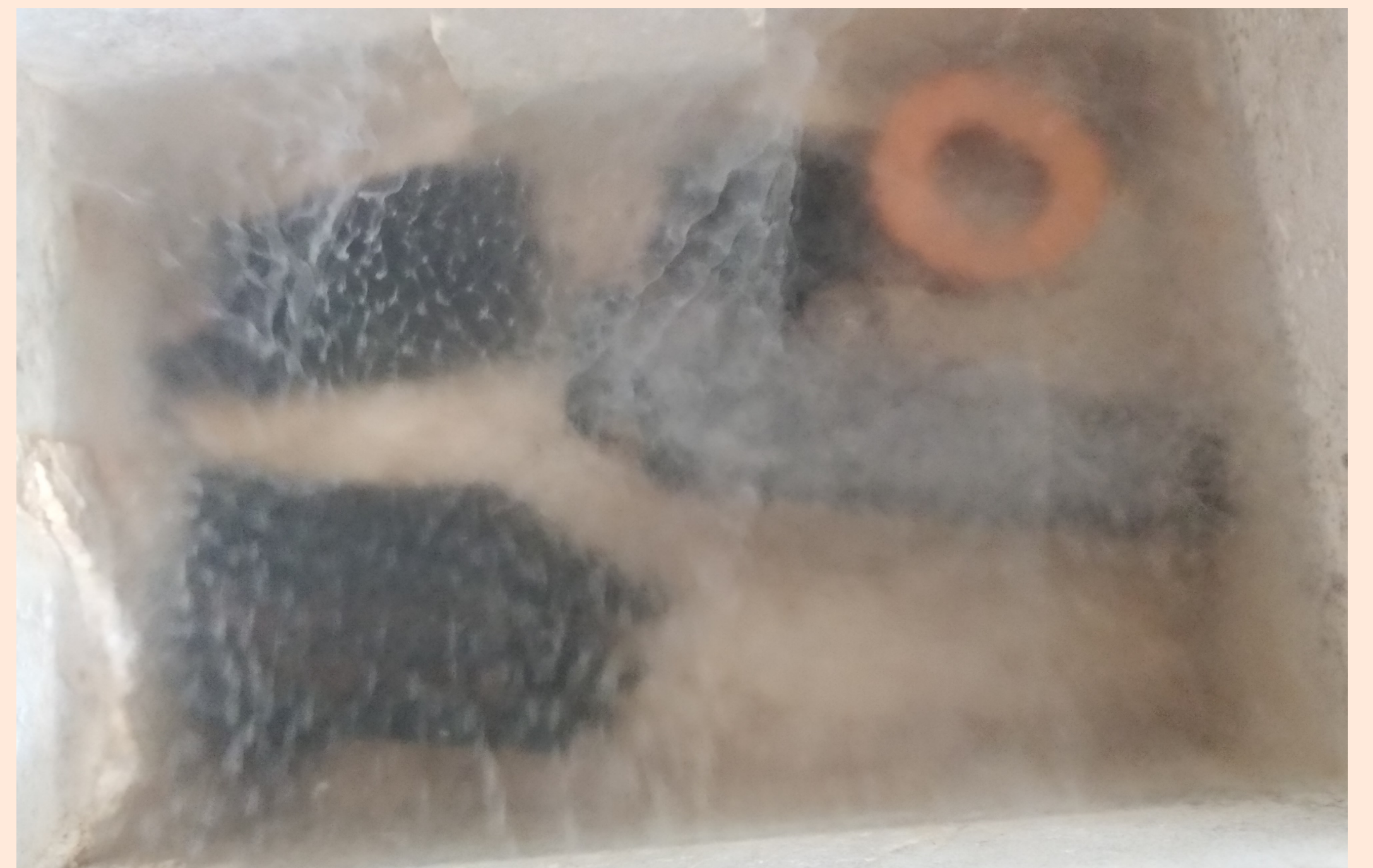
Photo 1. Cooling of tire samples in liquid nitrogen
