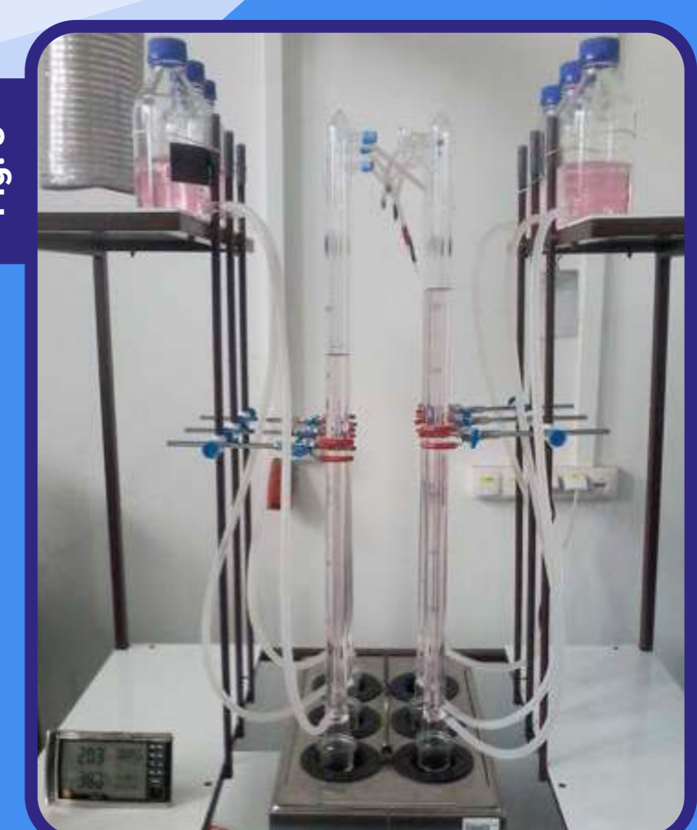
DIN 38414/8 eudiometric sets used for the experiments with anaerobic digestion of sewage sludges
