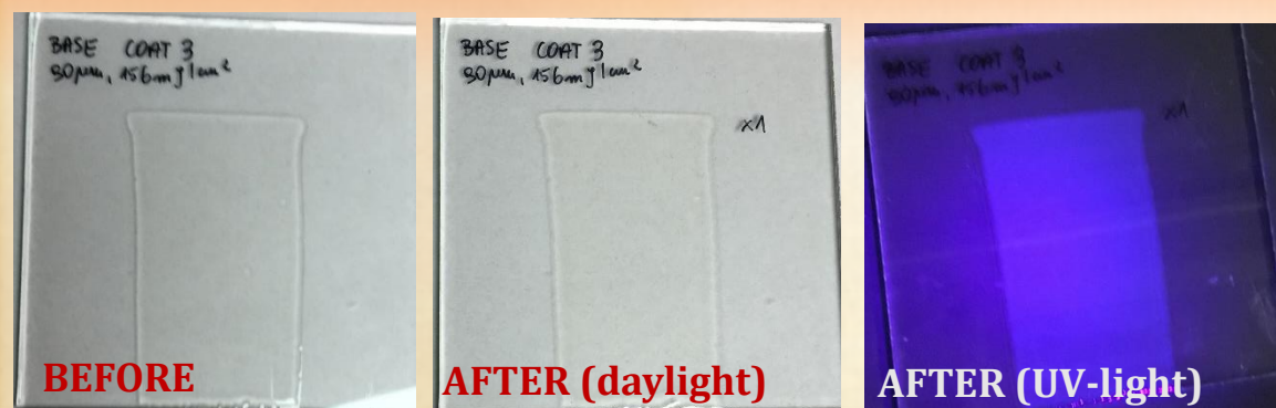
Fig. 1. Photographs of coatings obtained using the developed resins containing biphenyl derivatives as a component of the photoinitiating system.
